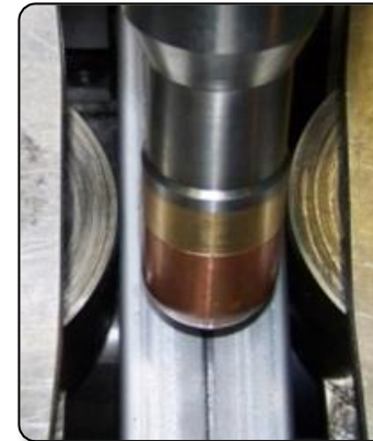
Examples of continuous longitudinal seam welding of hollow sections
